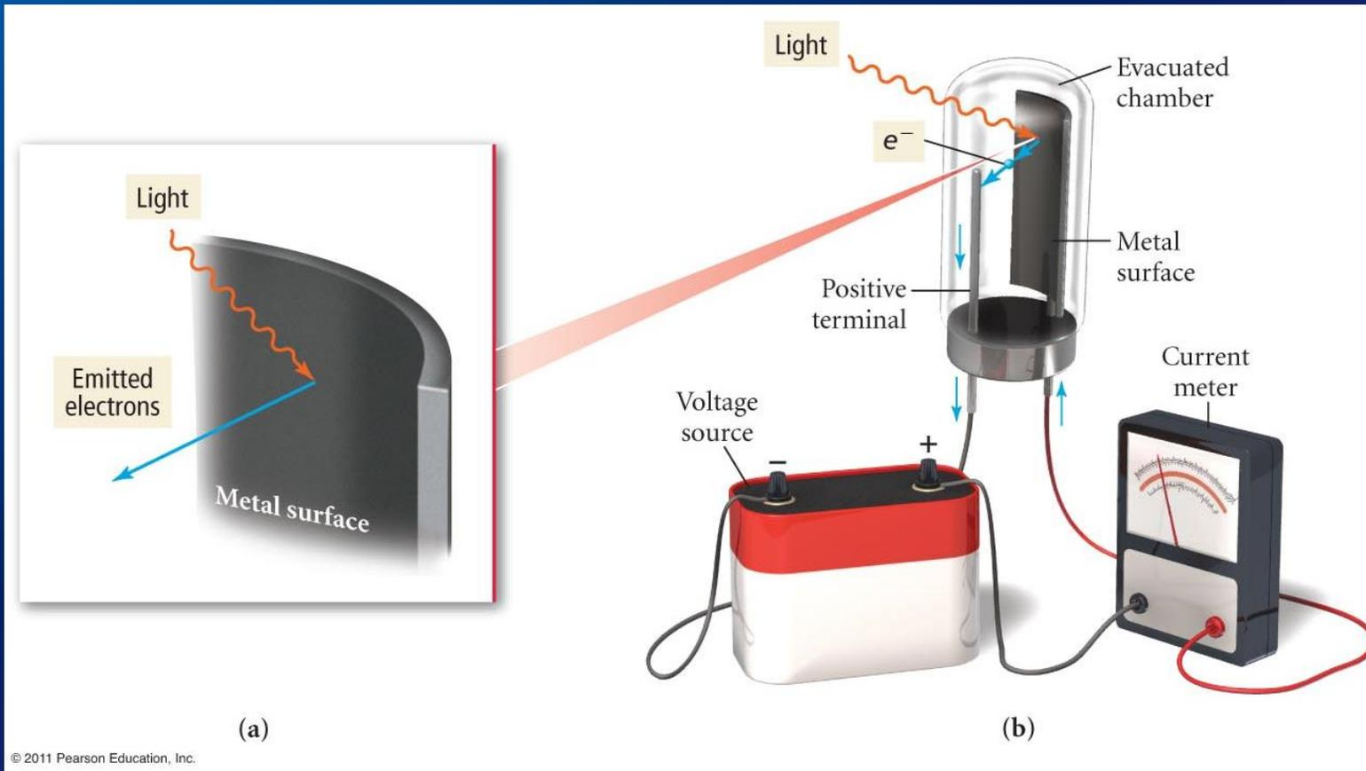
Evacuated tube containing metal sheet
